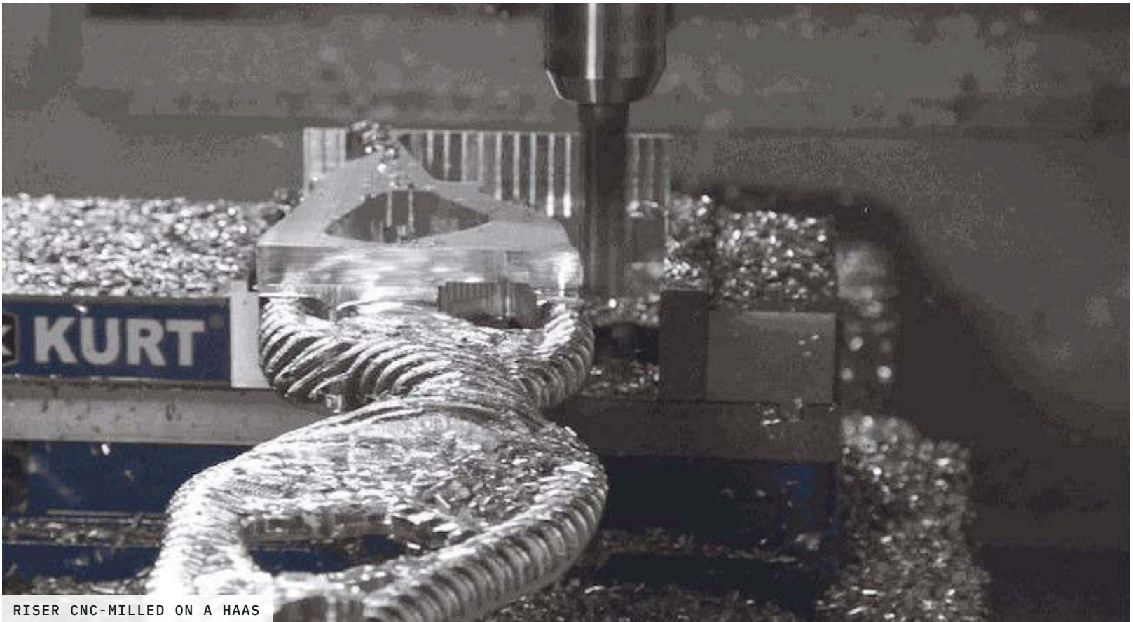
RISER CNC-MILLED ON A HAAS
